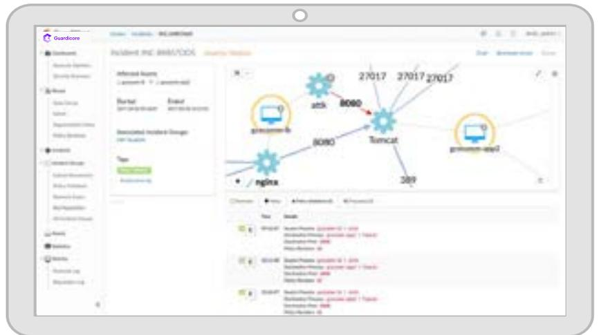
Guardicore Centra detects a potential breach via a segmentation policy violation involving an unauthorized process attempting to communicate on an authorized port between two permitted hosts.
